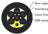
Bare copper conductor Polychloroprene rubber outer jacket Green/Yellow wire EPR insulation
